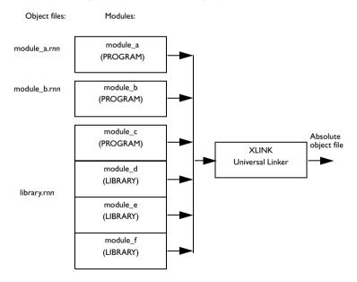
The main program has been assembled from two source files, module\_a.snn and module\_b.snn, to produce two relocatable files. Each of these files consists of a single module, module\_a and module\_b. By default, the assembler assigns the PROGRAM attribute to both module\_a and module\_b. This means that they will always be loaded and linked whenever the files they are contained in are processed by the IAR XLINK Linker.
