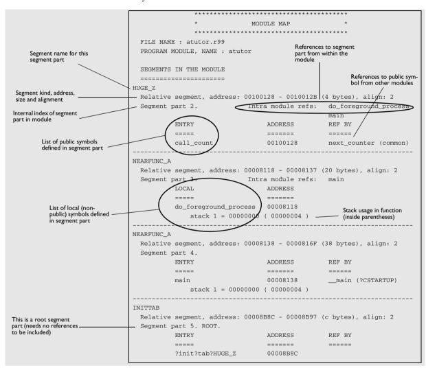
If the module contains any non-relocatable parts, they are listed before the segments.
