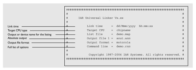
The full list of options shows the options specified on the command line. Options in command files specified with the -f option are also shown, in brackets.
