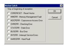
Figure 57: The Vector Catch dialog box—for ARM9/Cortex-R4 versus for Cortex-M3
