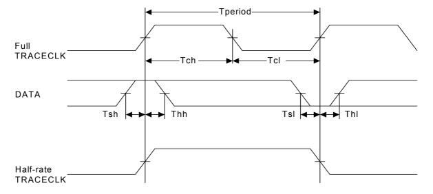
Note:J-Trace supports half-rate clocking mode. Data is output on each edge of the TRACECLK signal and TRACECLK (max) <= 100MHz. For half-rate clocking, the setup and hold times at the JTAG+Trace connector must be observed.
