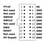
The J-Link and J-Trace JTAG connector is also compatible to ARM's Serial Wire Debug (SWD).
