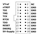
J-Link and J-Trace have a JTAG connector compatible to ARM's Multi-ICE. The JTAG connector is a 20 way Insulation Displacement Connector (IDC) keyed box header (2.54mm male) that mates with IDC sockets mounted on a ribbon cable.
