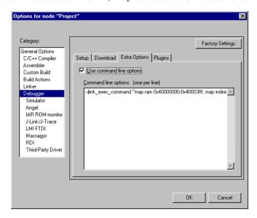
With these additional commands are the values of the fast GPIO registers in the C-Spy debugger correct and can be used for debugging. For more information about J-Link command line options refer to subchapter *Command strings* on page 65.
