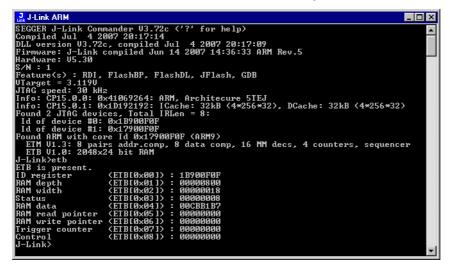
The result of the limited buffer size is that not more data can be traced than the buffer can hold. Through this limitation is an ETB not in every case an fully-fledged alternative to the direct access to an ETM via J-Trace.
