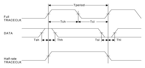
Note:J-Trace supports half-rate clocking mode. Data is output on each edge of the TRACECLK signal and TRACECLK (max) <= 100MHz. For half-rate clocking, the setup and hold times at the JTAG+Trace connector must be observed.
