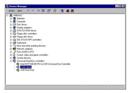
Right-click on the driver to open a context menu which contains the command **Properties**. If you select this command, a **J-Link driver Properties** dialog box is opened and should report: **This device is working properly**.
