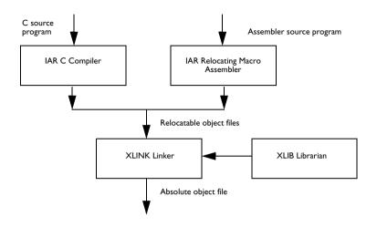
The following diagram illustrates the linking process:
