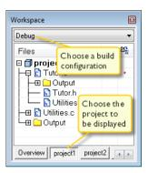
For each file that has been built, an Output folder icon appears, containing generated files, such as object files and list files. The latter is generated only if the list file option is enabled. The Output folder related to the project node contains generated files related to the whole project, such as the executable file and the linker map file (if the list file option is enabled).
