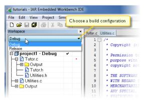
By default, the IDE creates two build configurations when a project is created—**Debug** and **Release**. Every build configuration has its own project settings, which are independent of the other configurations.
