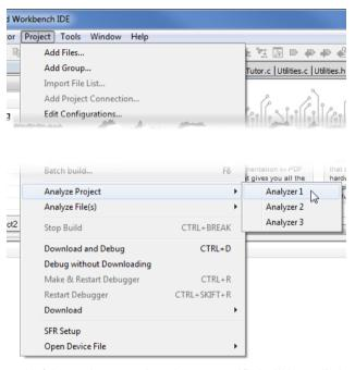
Each of the regular expressions that you specified will be applied on each line of output from the external analyzer. Output from the analyzer is listed in the Build Log window. You can double-click any line that matches the **Location** regular expression you specified in the **External Analyzer** dialog box to jump to the corresponding location in the editor window.
