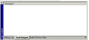
This window displays any messages output by user-defined tools in the **Tools** menu, provided that you have selected the option **Redirect to Output Window** in the **Configure Tools** dialog box; see *Configure Tools dialog box*, page 70. When opened, this window is, by default, grouped together with the other message windows.
