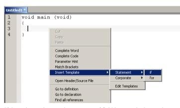
If the code template requires any type of field input, as in the for loop example which needs an end value and a count variable, an input dialog box appears.
