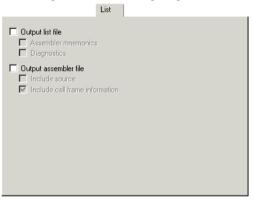
By default, the compiler does not generate a list file. Select any of the following options to generate a list file or an assembler file. The list file will be saved in the List directory, and its filename will consist of the source filename, plus the filename extension lst.
