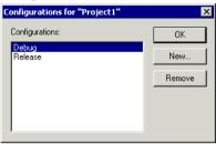
Use this dialog box to define new build configurations for the selected project; either entirely new, or based on a previous project.
