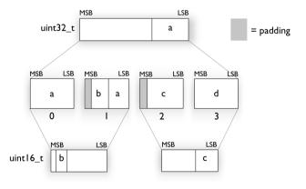
In big-endian mode, each bitfield is allocated starting from the most significant free bit of its container to ensure that it is placed into bytes from left to right.
