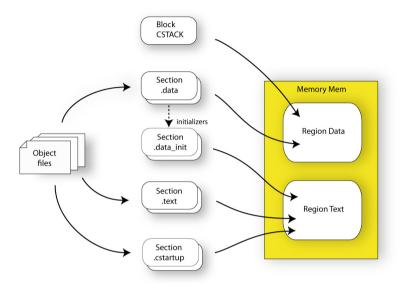
This illustration gives a schematic overview of how the application is placed in memory:
