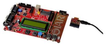
**l-jet** is an in-circuit debugging probe, which connects the chip's JTAG/SWD ports via USB to the host PC. I-jet integrates into IAR Embedded Workbench and is plug-and-play compatible.
