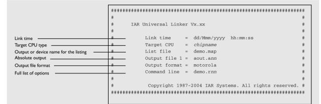
The full list of options shows the options specified on the command line. Options in command files specified with the -f option are also shown, in brackets.
