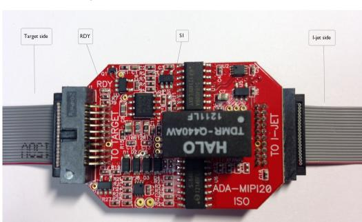
The adapter is automatically recognized by the C-SPY, and the adapter powers up and the green **RDY** LED is turned on.
