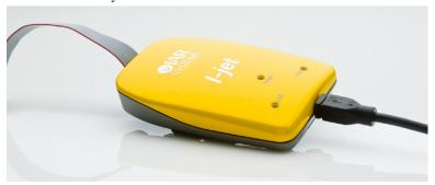
I-jet streams the program counter, variables, and power measurement data to the host
