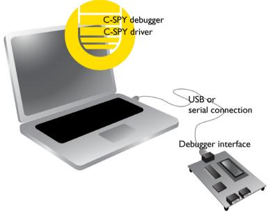
Using the C-SPY ROM-monitor driver, C-SPY can connect to various target hardware that have the ROM-monitor located in memory.
