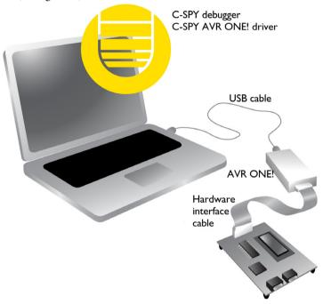
When a debugging session is started, your application is automatically downloaded and programmed into flash memory. You can disable this feature, if necessary.
