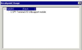
This window lists all breakpoints currently set in the target system, both the ones you have defined and the ones used internally by C-SPY. The format of the items in this window depends on the C-SPY driver you are using.
