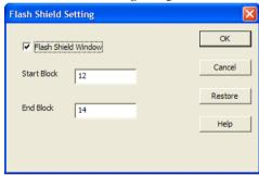
By default, the entire flash memory is write-protected by a *flash shield*. Use this dialog box to specify that a range of memory blocks can be modified by the flash self-programming. This memory range is called a *flash shield window*.
