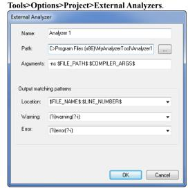
Use this dialog box to configure the invocation of the external analyzer that you want to add to the standard build toolchain.
