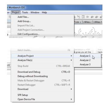
Each of the regular expressions that you specified will be applied on each line of output from the external analyzer. Output from the analyzer is listed in the Build Log window. You can double-click any line that matches the **Location** regular expression you specified in the **External Analyzer** dialog box to jump to the corresponding location in the editor window.
