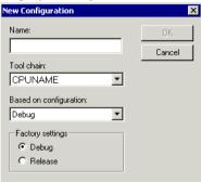
Use this dialog box to define new build configurations; either entirely new, or based on any currently defined configuration.
