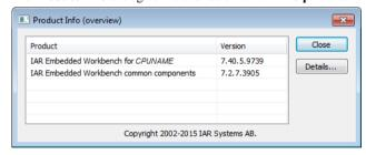
This dialog box lists the version number of your IAR Embedded Workbench product installation and the shared components. Note that the initial digit of the version number of the shared components (in this screen shot 7) is reflected by the default installation directory x:\Program Files\IAR Systems\Embedded Workbench 7.n\.
