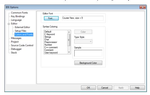
Use this page to specify the colors and fonts used for text in the editor windows. The keywords controlling syntax highlighting for assembler and C or C++ source code are specified in the files syntax\_icc.cfg and syntax\_asm.cfg, respectively. These files are located in the 78K\config directory.
