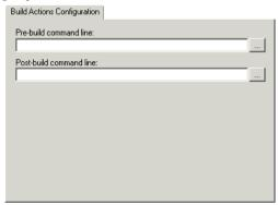
If a pre- or post-build action returns a non-zero error code, the entire **Build** or **Make** command is aborted.
