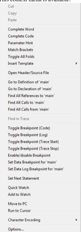
The contents of this menu depend on whether the debugger is started or not, and on the C-SPY driver you are using. Typically, additional breakpoint types might be available on this menu. For information about available breakpoints, see the *C-SPY® Debugging Guide for 78K*.
