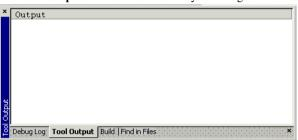
This window displays any messages output by user-defined tools in the **Tools** menu, provided that you have selected the option **Redirect to Output Window** in the **Configure Tools** dialog box; see *Configure Tools dialog box*, page 66. When opened, this window is, by default, grouped together with the other message windows.
