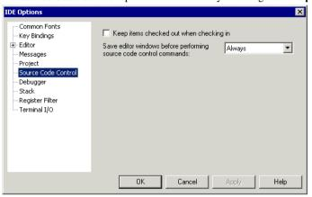
Use this page to configure the interaction between an IAR Embedded Workbench project and an SCC project.
