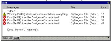
This window displays the messages generated when building a build configuration. When opened, the window is, by default, grouped together with the other message windows. Double-click a message in the **Build** window to open the appropriate file for editing, with the insertion point at the correct position.
