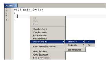
If the code template requires any type of field input, as in the for loop example which needs an end value and a count variable, an input dialog box appears.
