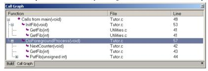
This window displays calls to or calls from a function. The window is useful for navigating between the function calls.
