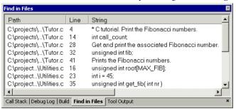
This window displays the output from the Edit>Find and Replace>Find in Files command. When opened, this window is, by default, grouped together with the other message windows.
