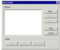
This dialog box lists all defined batches of build configurations. For more information, see *Building multiple configurations in a batch*, page 112.
