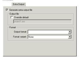
For *some* debugger systems, two output files from the same build process are required—one with the necessary debug information, and one that you can burn to your hardware before debugging. This is useful when you want to debug code that is located in non-volatile memory.
