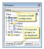
For each file that has been built, an Output folder icon appears, containing generated files, such as object files and list files. The latter is generated only if the list file option is enabled. The Output folder related to the project node contains generated files related to the whole project, such as the executable file and the linker map file (if the list file option is enabled).
