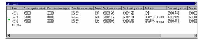
The currently active task is indicated by an arrow in the first column, pointing to the task currently running. The last row of the Task window is always NO TASK. When the arrow points to NO TASK execution is taking place outside any task, in the scheduler etc.
