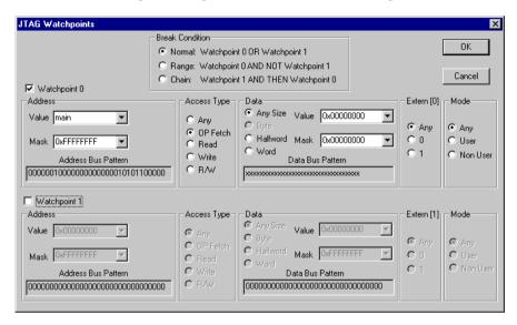
Use this dialog box to directly control the two hardware watchpoint units. If the number of needed watchpoints (including implicit watchpoints used by the breakpoint system) exceeds two, an error message will be displayed when you click the **OK** button. This check is also performed for the C-SPY **Go** button.
