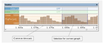
The power graph displays a graphical view of power measurement samples generated by the debug probe or associated hardware in relation to a common time axis.
