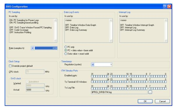
Use this dialog box to configure the serial-wire output communication channel and the hardware's generation of trace data.
