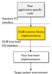
For example, if your application calls the functions printf and fputc in the standard I/O interface, the implementations of those functions both call the low-level function \_\_write to output individual characters. To make them work, you just need to provide an implementation of the \_\_write function—either by implementing it yourself, or by using a third-party implementation.
