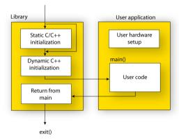
• Static and global variables are initialized. That is, zero-initialized variables are cleared and the values of other initialized variables are copied from ROM to RAM memory. This step is skipped if \_\_low\_level\_init returns zero. For more information, see *Initialization at system startup*, page 94.
