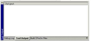
The Tool Output window displays any messages output by user-defined tools in the **Tools** menu, provided that you have selected the option **Redirect to Output Window** in the **Configure Tools** dialog box; see *Configure Tools dialog box*, page 64. When opened, this window is, by default, grouped together with the other message windows.
