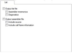
By default, the compiler does not generate a list file. Select any of the following options to generate a list file or an assembler file. The list file will be saved in the List directory, and its filename will consist of the source filename, plus the filename extension lst.
