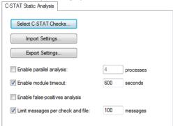
Use this page to specify options for performing a static analysis using C-STAT.
