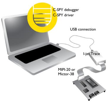
I-jet Trace streams the program counter, variables, and power measurement data to the host computer to provide a view into program execution in real time. Besides the typical JTAG debugging, I-jet Trace is capable of providing power to the target board, and measuring it with sufficient accuracy to provide a power profile during program execution in real time. This feature is referred to as *power debugging*.
