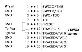
The mating connector for a target board has the pitch size 0.05 in (1.27 mm). You can, for example, use part number SHF-110-01-L-D.
