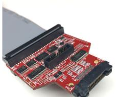
The mating connector for Mictor-38 on target board is AMP/Tyco 5767054-1.
