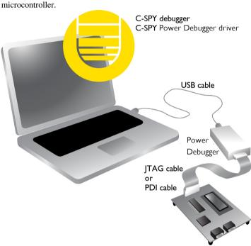
interface—for example JTAG, PDI, debugWIRE, ISP, TPI, or UPDI—on the microcontroller
