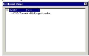
This window lists all breakpoints currently set in the target system, both the ones you have defined and the ones used internally by C-SPY. The format of the items in this window depends on the C-SPY driver you are using.
