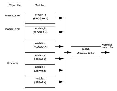
The main application has been assembled from two source files, module\_a.snn and module\_b.snn, to produce two relocatable files. Each of these files consists of a single module, module\_a and module\_b. By default, the assembler assigns the PROGRAM attribute to both module\_a and module\_b. This means that they will always be loaded and linked whenever the files they are contained in are processed by the IAR XLINK Linker.
