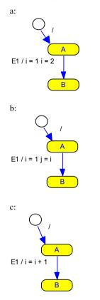
Multiple assignments to the same variable result in an ambiguity. An example of that is system a because i is assigned to twice on the same transition. The systems b and c are unambiguous because the buffered value of i is read in the assignments j = i or i = i + 1, respectively.
