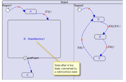
This figure shows state B after it has been converted to a submachine state; the submachine state has been automatically associated with the state machine template:
