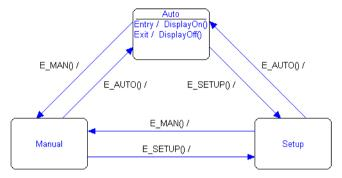
In the following diagram, the entry and exit reactions are placed on the individual transitions, giving a more complex graphical model:
