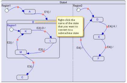
This is an example state machine before changing a state to a submachine state:
