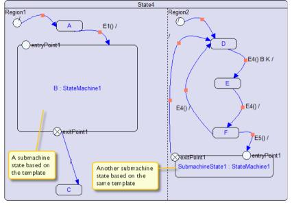
This example shows a state machine model where two submachine states are instances of the template, The example also shows the entry and exit states reference points:
