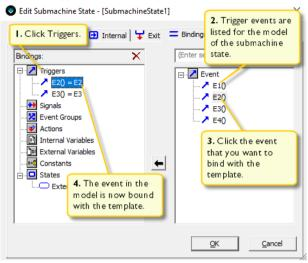
Now the state machine template is instantiated in two places—two different instances. They do not work the same, because they have different bindings. So even though the model uses the same template in two places, the two instances work differently.
