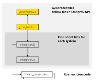
In the figure, the rectangle in yellow represents the header files that are part of the API. The arrows in the figure indicate how the header files are included in the source files. There must be a user-written source file for each system. As can be seen in the figure, each such file must include all project header files and all system header files for a specific system.
