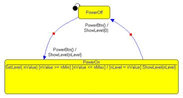
Switching from state to state is done by triggering the event PowerBtn. When the state machine is in the PowerOn state, an internal reaction can be triggered by the event SetLevel. This internal reaction calls the action ShowLevel that can be used for displaying the event parameter from SetLevel.
