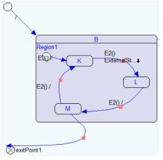
This figure shows the automatically created state machine template based on the original state B:
