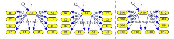
Treating state configurations symbolically can make verification of systems with large state spaces possible:
