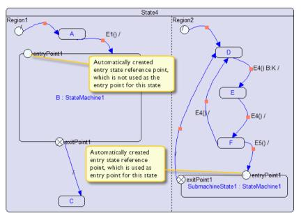
In this example, the entry point reference state is used as entry point in one of the template instances, but not in the other.
