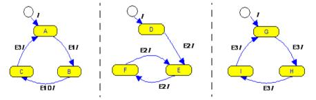
The first machine deadlocks when the system enters the state configurations (B, F) and (B, E).
