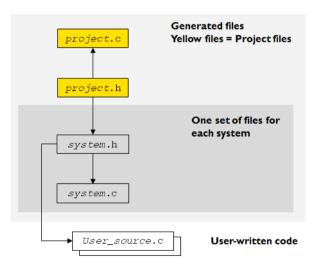
In the figure, the dark gray area represents the source and header files that are part of the API. The arrows in the figure indicate how the header files are included in other files. *System* stands for the system name. The generated API files are the same for C and C++ code (with the appropriate filename extension) and for table-based and readable code.
