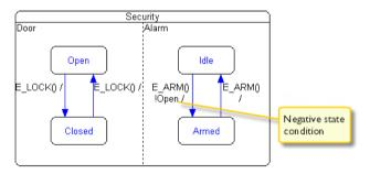
In this case, the state condition is negative in that the door must *not* be in the state Open. This is specified by the expression ! Open on the transition from the state Idle to the state Armed. This transition will only go to the state Armed if the state machine Door is not in the state Open.
