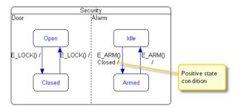
transition fire. This figure illustrates an example of a positive state condition in a security system:
