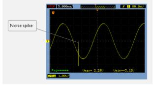
Power debugging will help you investigate interference from digital and power supply lines into the analog parts. Power spikes in the vicinity of AD conversions could be the source of noise and should be investigated.
