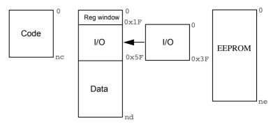
four address zones—CODE, DATA, EEPROM, and IO\_SPACE—in the debugger cover the whole AVR memory range.
