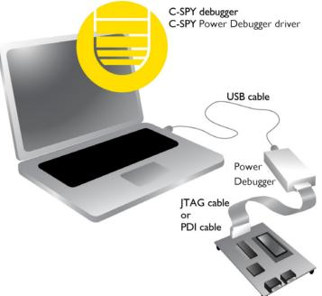
interface—for example JTAG, PDI, debugWIRE, ISP, TPI, or UPDI—on the microcontroller.
