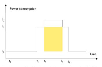
At  $t_1$ , the system is activated whereby the current rises to  $I_1$  which is the system's power consumption in active mode when at least one peripheral device turned on, causing the
