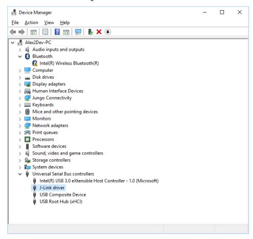
Right-click on the driver to open a context menu which contains the command Properties. If you select this command, a J-Link driver Properties dialog box is opened and should report: This device is working properly.
