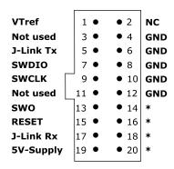
The J-Link and J-Trace JTAG connector is also compatible to ARM's Serial Wire Debug (SWD).
