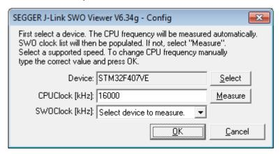
When running in normal mode J-Link SWO Viewer automatically performs the necessary initialization to enable SWO output on the target, in GDB Server mode the initialization has to be done by the debugger. Should you have a target connection already open e.g. a debug session in your IDE we recommend defining the parameters device name, CPU clock frequency and SWO clock frequency via CL to avoid connection errors.
