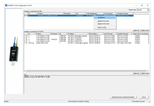
In order to configure an old J-Link, which uses the old USB 0 - 3 USB identification method, to use the new USB identification method (reporting the real serial number) simply select "Real SN" as USB identification method and click the OK button. The same dialog also allows configuration of the IP settings of the connected J-Link if it supports the Ethernet interface.
