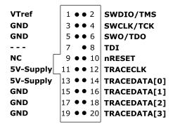
J-Trace provides a JTAG/SWD+Trace connector. This connector is a 19-pin connector (0.05" / 1.27mm). It connects to the target via an 1-1 cable.
