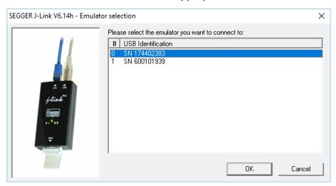
So even in IDEs which do not have an selection option for the J-Link, it is possible to connect to different J-Links.
