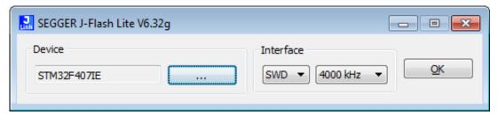
The main window of J-Flash Lite only consists of a few dialog elements that allow programming of the target:
