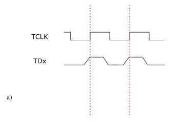
Drawing a) shows the correct behavior of a target and b) shows a target that does not apply setup times. Therefore in b) the undelayed signal TDx would be sampled as a logical 0 at the rising edge of TCLK which would give the J-Trace wrong tracing information. In the case where the sample point of TDx is moved to the left (negative) by  $\Delta t_d$  at each rising TCLK edge a logical 1 is sampled which in this case means that the J-Trace now receives the correct trace information.
