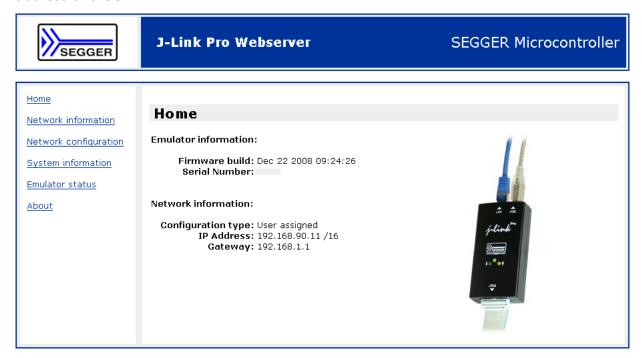
The Network configuration page allows configuration of network related settings (IP address, subnet mask, default gateway) of J-Link. The user can choose between automatic IP assignment (settings are provided by a DHCP server in the network) and manual IP assignment by selecting the appropriate radio button.
